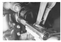
3/4 Use a strap wrench to loosen filter ...
