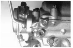
9/131 Align marks and tighten bolt
