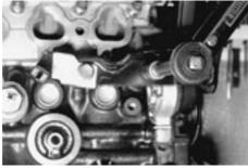
9/139 Torque tighten bracket bolts.
