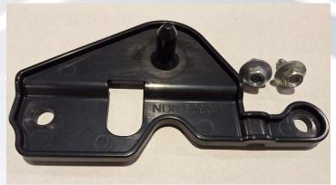
8. Assemble the holder (E) with the original screws. Then press the original retaining rubber into the opening provided on the underside of the air filter housing and install the original vibration damper rubber with sleeve.
