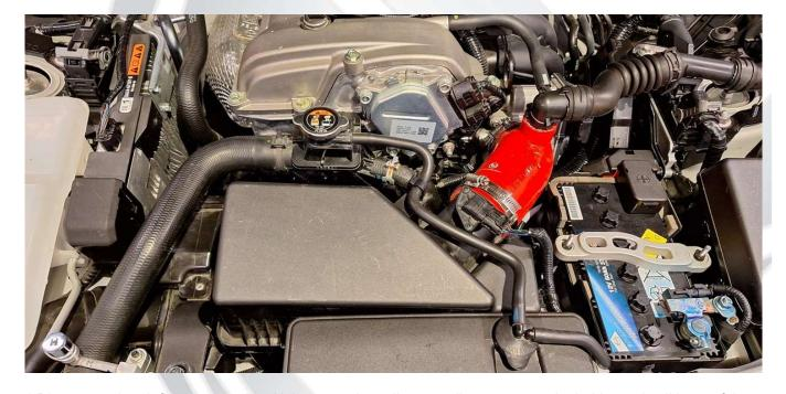
1.Disconnect the air flow sensor plug. Using curved needle nose pliers, squeeze the holder and pull it out of the holder.
